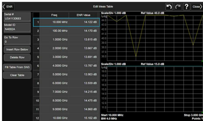
Automatically downloads ENR data from an SNS Series noise source into any NFA Series or any X-Series signal analyzer
